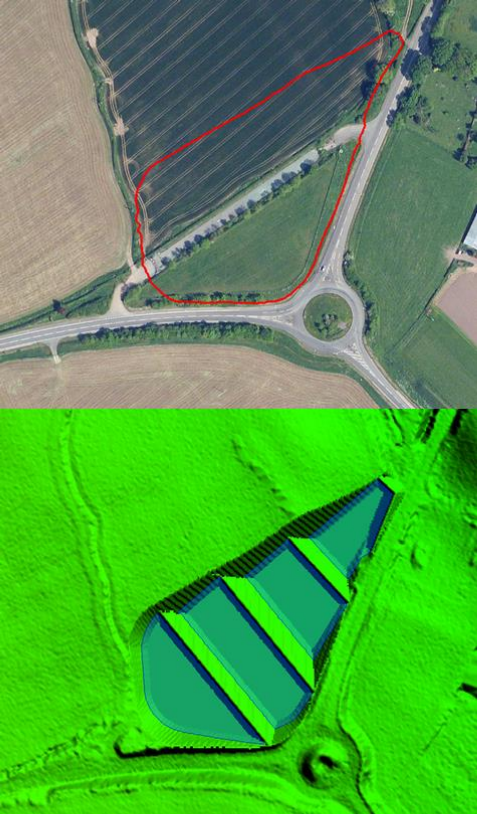
Figure 15: Ruthin Road attenuation storage area
